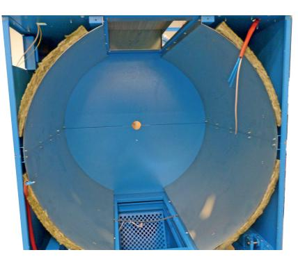
Drying area thermally and acoustically insulated with stone wool
